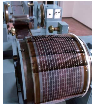
Production line for amorphous silicon solar cells, whose distinguishing feature is the roll-to-roll process
