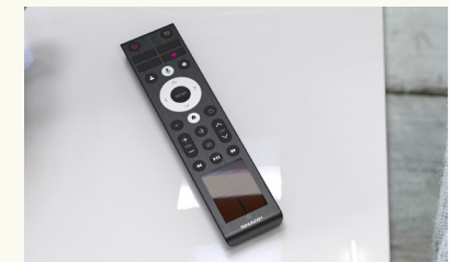
TV remote control with built-in solar panel
