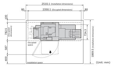
The above illustration indicates the Digital Multifunctional System BP-1250M model with the bypass tray and finisher installed.
