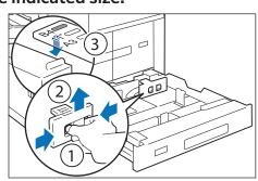
4. Pinch the guide clip(s) and adjust to the correct paper size.
