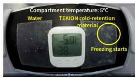
At a compartment temperature of 5°C, 10°C TEKION cold-retention material starts to freeze.
