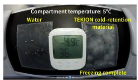
At a compartment temperature of 5°C, water undergoes no change, but TEKION cold-retention material freezes.
