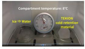
At a compartment temperature of 8°C, normal ice melts into water but 10°C TEKION cold-retention material remains in ice form.
