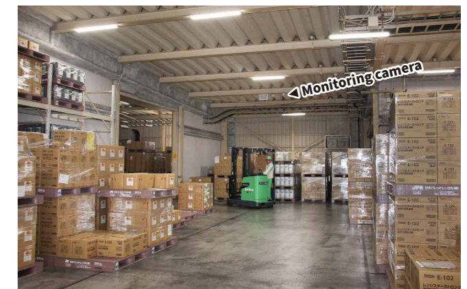
The monitoring cameras detect motion and automatically adjust lighting, even in large spaces with high ceilings.
