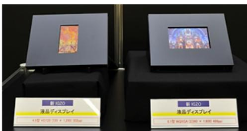
LCD panels incorporating IGZO oxide semiconductor technology
