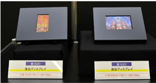
LCD panels incorporating IGZO oxide semiconductor technology
