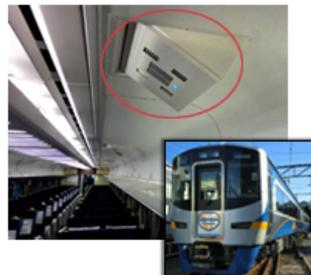
Plasmacluster ion generators are installed in the express trains of the Nankai Electric Railway Co., Ltd.
