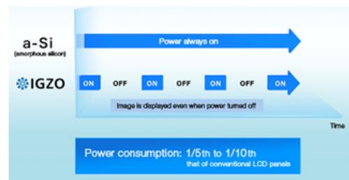
Comparison of energy consumption between Sharp's conventional a-Si LCD panel and the IGZO LCD panel
