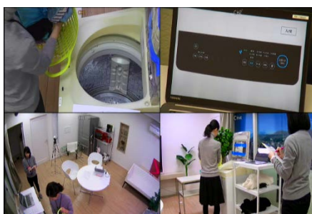
Conducting a usability test on a washing machine
