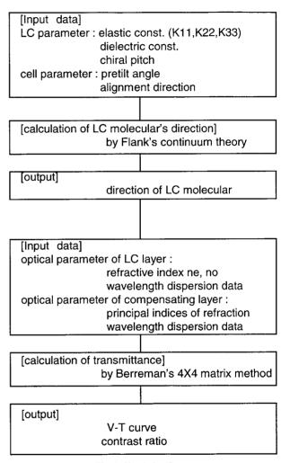
Fig. 1 Simulation flow.
