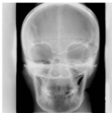
Fig. 12 X-ray image of a head phantom (9" a-Se).
