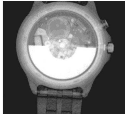
Fig. 10 X-ray image of a watch (3" CdTe).
