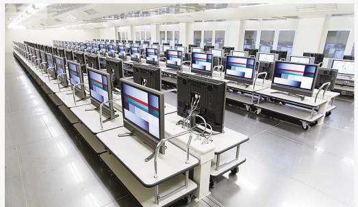
LCD TV production line (isothermal test process)
