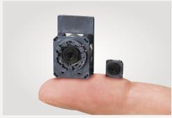
CCD (left) and CMOS (right) camera modules for mobile phones
