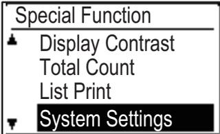
**Press the [SPECIAL FUNCTION] key (Fn), and select "System Settings" with the [▼] or [▲] key and press the [OK] key.**
