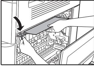
Open the fusing paper guide by pressing down the green-labelled projection on the guide and remove the misfed paper.
