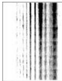
“Vertical dark streaks with print missing” on page 154
