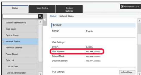
Scroll the screen down and check "IPv4 Address" in IPv4 Settings of TCP/IP.
