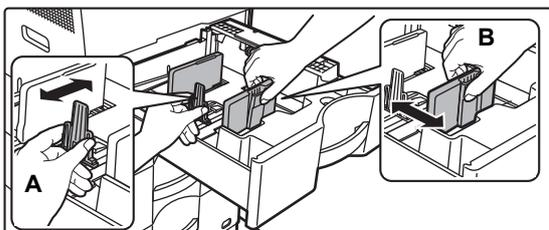
**Adjust guide plates A and B to match the longitudinal and transversal dimensions of the paper to be loaded.**
