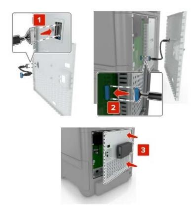
7 Reattach the controller board access cover.
