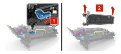
Note: The black imaging unit includes the black developer unit and photoconductor unit.
