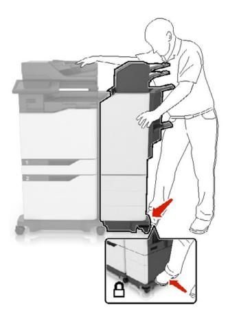
**14** Push the finisher to the printer by applying pressure at the bottom of the finisher until it *clicks* into place.
