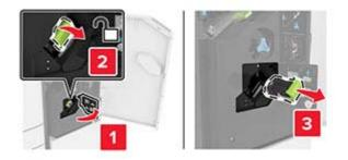
**3** Open the staple guard, and then remove the loose staples.
