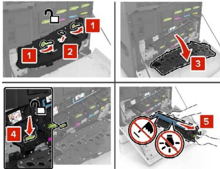
4 Remove the photoconductor unit.
