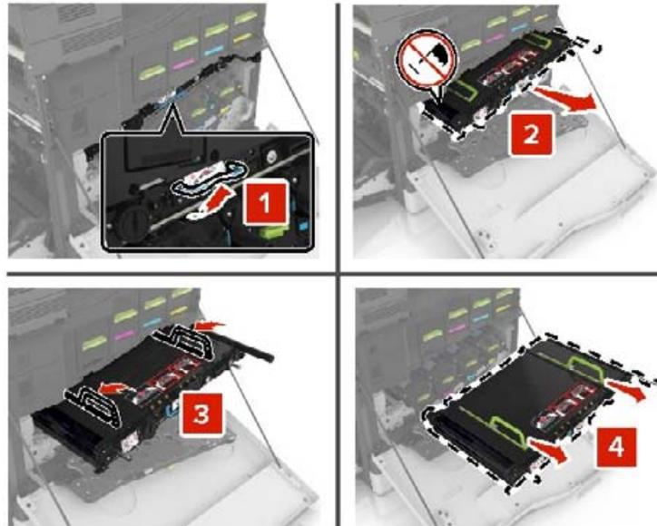
**6** Unpack the new transfer belt, and then remove the packing material.
