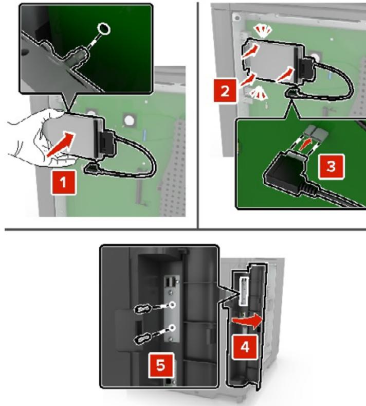
If an internal solutions port (ISP) is installed, then do the following:
