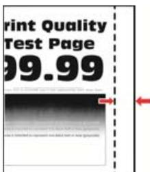
**Note:** Before solving the problem, print the Print Quality Test Pages. From the control panel, navigate to **Settings > Troubleshooting > Print Quality Test Pages**. For non-touch-screen printer models, press
