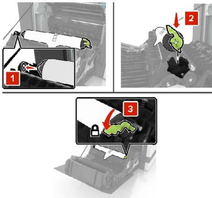
**5** Remove the white packing material.
