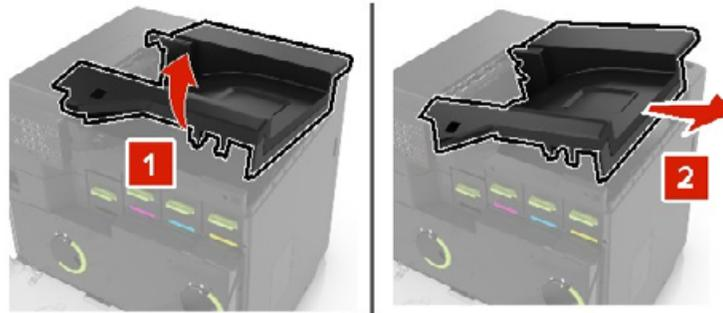
5 Unpack the staple finisher, and then remove the packing material.
