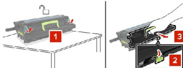
**5** Unpack the new developer unit, and then remove the packing material.
