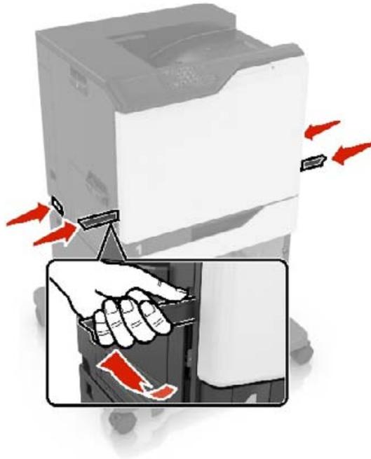
**Note:** If optional trays are already installed, then unlock them from the printer before lifting the printer. Do not try to lift the printer and trays at the same time.
